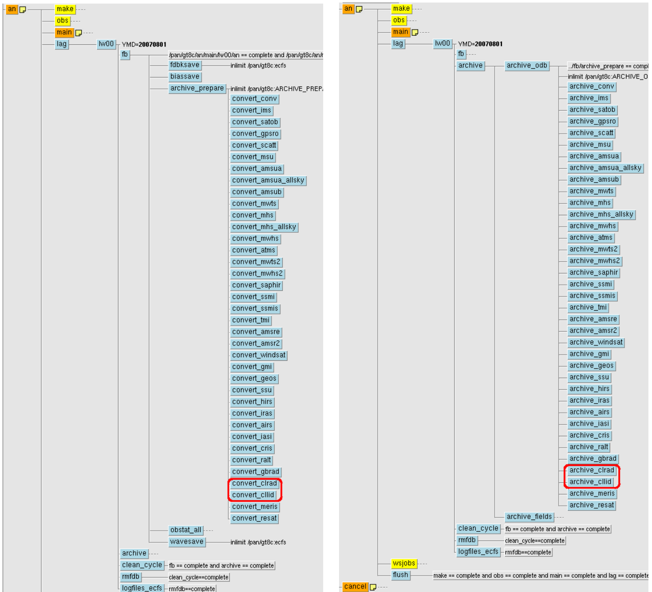
Figure 3.7: Post-processing tasks in 4D-Var cycling: (left) creation of ODB database with direct column access under archive_prepare task group - tasks convert_clrad and convertcllid (marked in red) used for the new cloud radar and lidar observations; (right) archiving ODB database under archive_odb task group - tasks archive_clrad and archive_cllid (marked in red) for the new observations.
