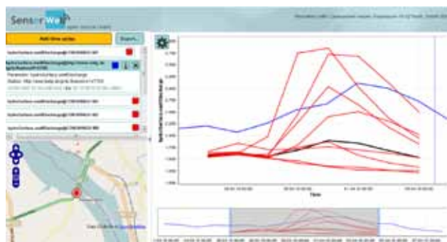
Figure 7 Example of the web service run by 52° North showing some randomly selected ensemble members from TIGGE discharge forecasts for a point on the Susquehanna River in Maryland, US.
