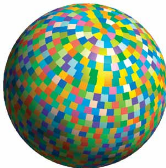
Figure 3 Equal region domain decomposition with 1,600 partitions for the N1280 octahedral reduced Gaussian grid (see right-hand panel in Figure 2).
