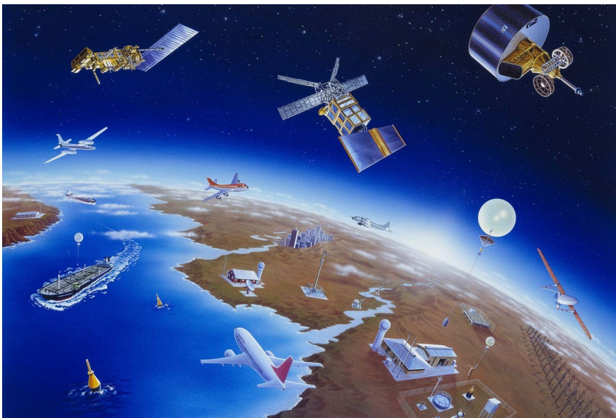
Figure 1 The WMO Integrated Global Observing System (WIGOS) combines the observing capabilities of surface- and space-based platforms and stations to serve a variety of weather and climate needs. ( Graphic: WMO )
