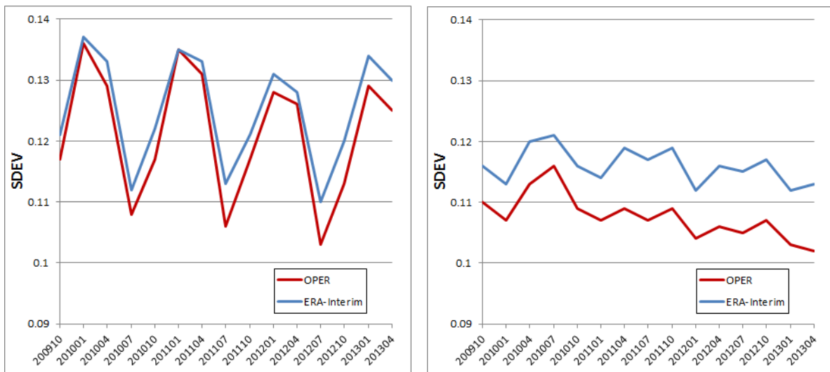
Figure 29: Seasonal averages of the day 3 forecast error standard deviation of normalized TOA reflected solar flux (daily totals) in the parts of the northern hemisphere extratropics (left panel) and tropics (right panel) which are covered by the CM-SAF product in Figure 28.
