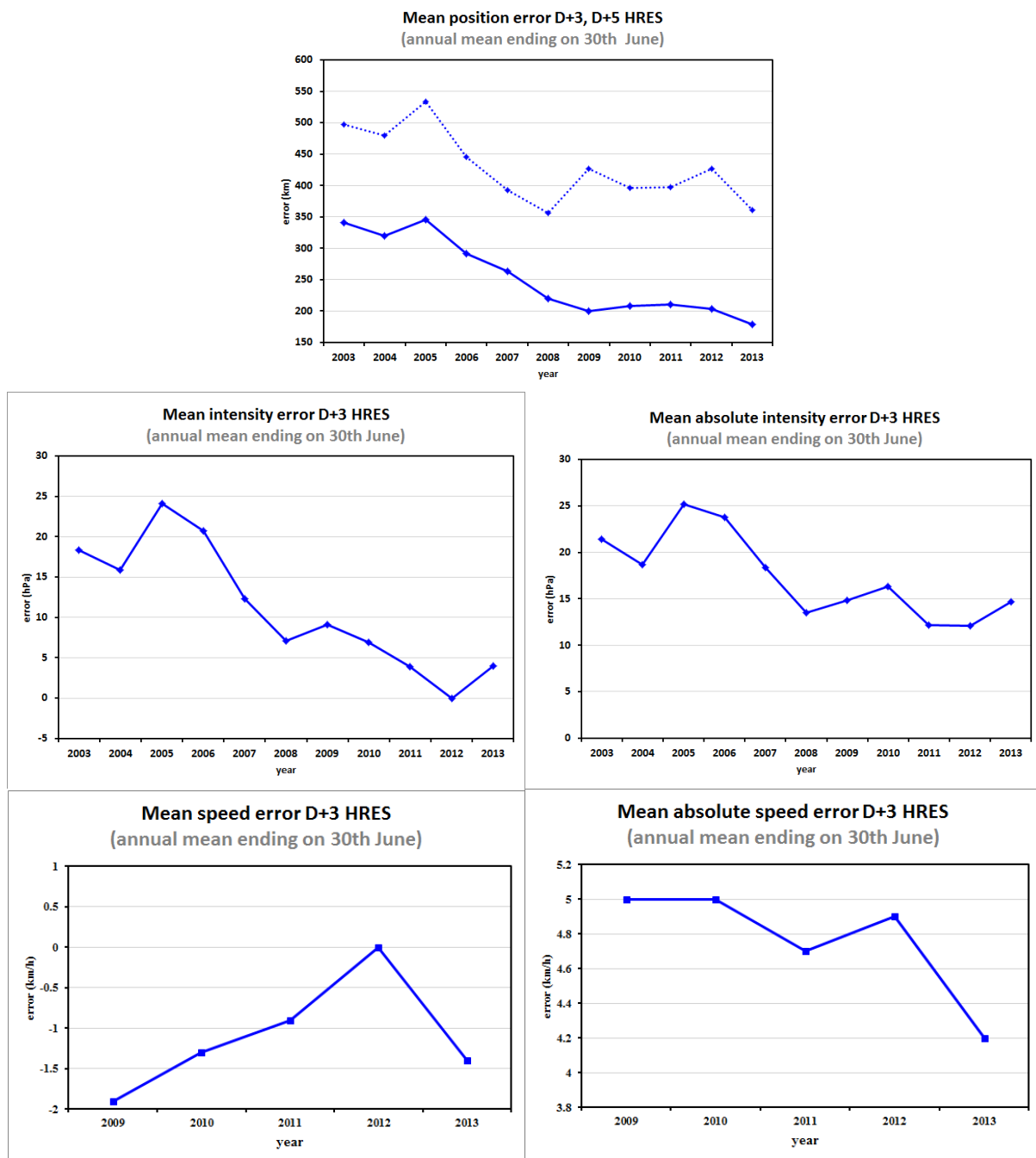
Figure 35: Verification of tropical cyclone predictions from the operational high-resolution forecast. Results are shown for all tropical cyclones occurring globally in 12-month periods ending on 30 June. Verification is against the observed position reported in real time via the GTS. Top left: supplementary headline score – the mean position error (km) of the three-day high-resolution forecast. The error for day 5 is included for comparison. Centre left: mean error (bias) in the cyclone intensity (difference between forecast and reported central pressure); positive error indicates the forecast pressure is less deep than observed. Centre right: mean absolute error of the intensity. Bottom left: mean speed error; negative values indicate the forecast is too slow compared to the observed cyclones. Bottom right: mean absolute error of the speed.
